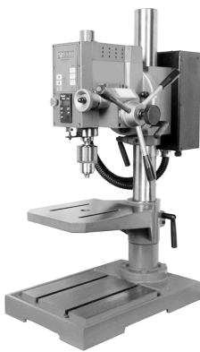
Fig.6-9 Sensitive Drill Press
